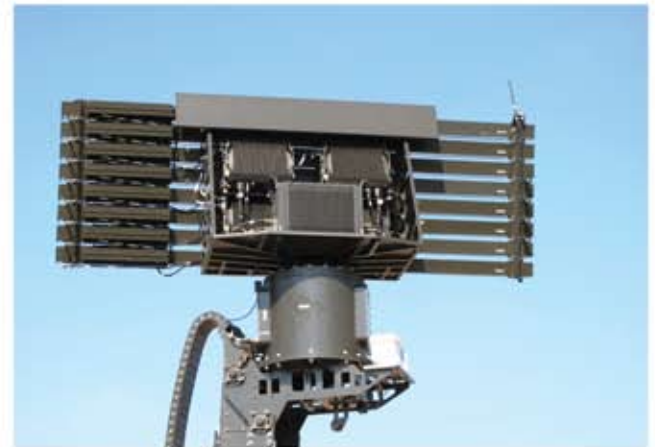
ELM-2106 ATAR antenna back side with T/R units and IFF
