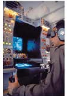
Boom Operator Station
