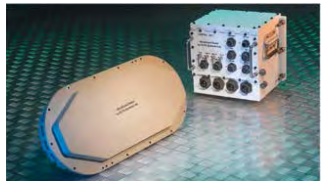
Typical Radar Antenna and Central Unit
